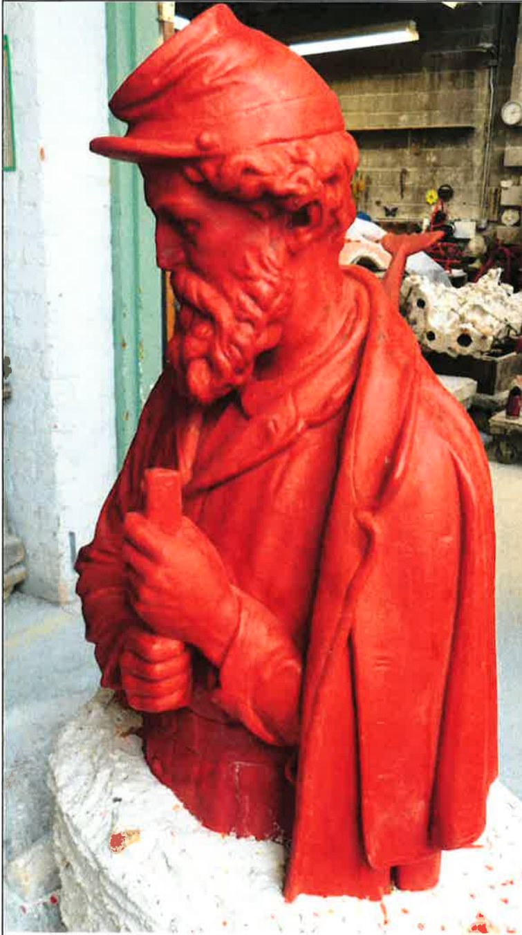
Wax cast from the rubber mold for “lost Wax” casting process. The wax will have sprues added and then encased in plaster.
